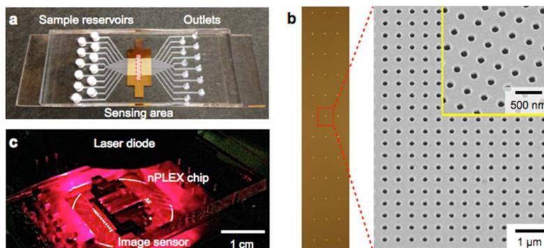
**Fig. 6. First nPLEX prototype**
