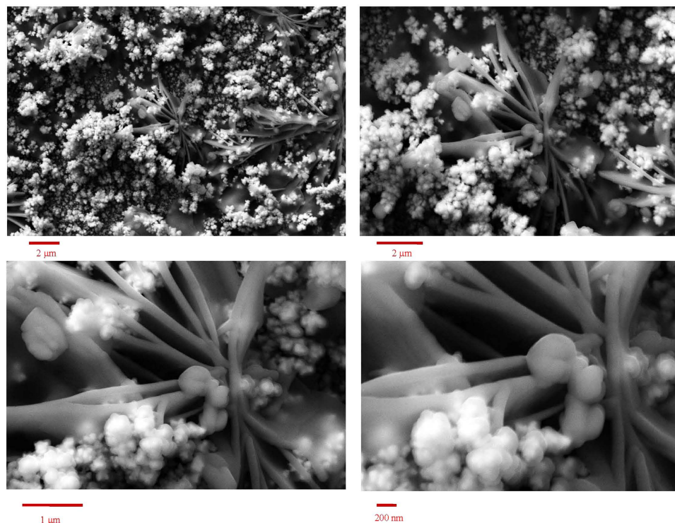
Figure 1. FESEM images of gold nanoribbons covered by gold nanoblooms with different magnifications.
