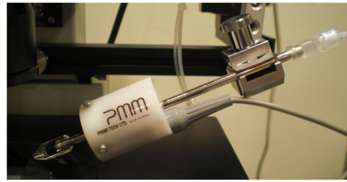
Fig. 2 Drive unit of a Piezo-micromanipulator (MB-U, PRIME TECH Ltd., Japan) attached to the micropipette holder
