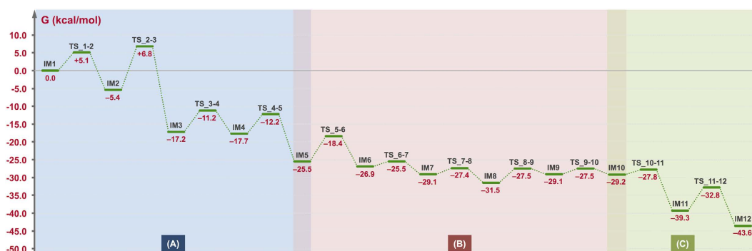
Figure 3. Computed potential energy profiles for the “cation-stitching cascade” reaction. Potential energies (kcal/mol, Gibbs free energies calculated at the M062X/6-31G** level) relative to IM1 are shown in red.
