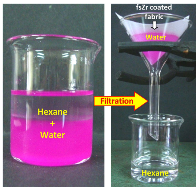
Figure 6. Image showing the separation process for hexane-water mixture. Hexane freely permeated and rapidly accumulated into the bottom of the beaker through the fsZr coated superhydrophobic/superoleophilic cotton fabric whereas water (dyed with Rhodamine B) still remained on the textile surface.
