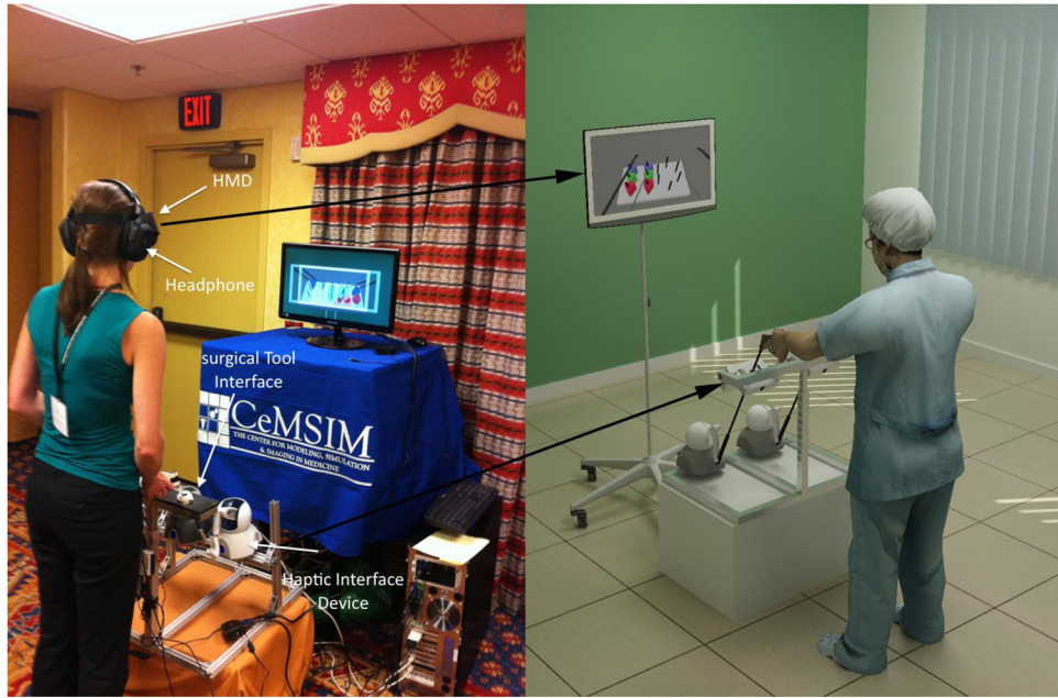
Figure 1. The Gen2-VR© simulator showing the physical interface (left) and the immersive virtual environment (right) with the user represented as an avatar.
