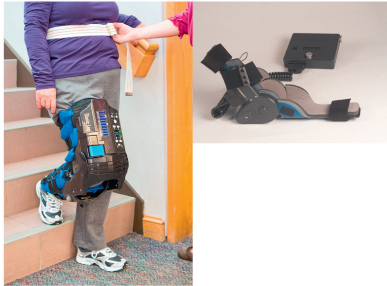
Fig. 23.3. Myomo e100 and Tybion. They can actuate the elbow and knee of stroke patients. (Courtesy Tybion and J. Stein, Department of Rehabilitation and Regenerative Medicine, Columbia University and Division of Rehabilitation Medicine, Weill Cornell Medical College.)
