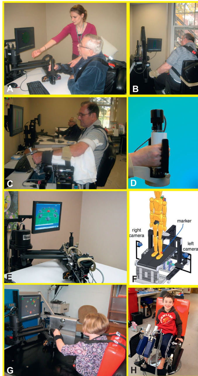
Fig. 23.5. MIT Gym of Robots (commercialized by Interactive Motion Technologies, Watertown, MA). (A) MIT-Manus to promote neurorecovery of the injured brain and control of the shoulder and elbow segments; (B) the antigravity to promote training of the shoulder against gravity. (C) The wrist robot which affords training of the 3 degrees of freedom of the wrist and forearm; (D) the hand module for grasp and release. (E) The combination of shoulder and elbow robot with the wrist module mounted at the tip of first affording training for both transport of arm and object manipulation; (F) a sketch of the alpha-prototype of the MIT-
