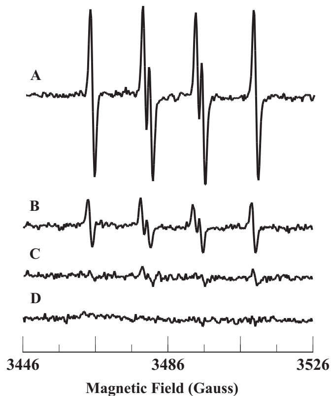
Fig. 3. Room temperature EPR spectra of the sulfite radical adduct of DMPO, \text{DMPO}\text{-SO}_3^- . All the reactions were performed in 50 mM phosphate buffer (pH=7.4) containing 0.1 mM DTPA. Spectrum A: DMPO (0.1 M), \text{Fe}^{3+} cyt c (0.1 mM), sulfite (0.5 mM), and \text{H}_2\text{O}_2 (0.1 mM). Spectrum B: DMPO (0.1 mM), sulfite (0.5 mM), and \text{H}_2\text{O}_2 (0.1 mM). Spectrum C: DMPO (0.1 M), \text{Fe}^{3+} cyt c (0.1 mM), and sulfite (0.5 mM). Spectrum D: DMPO (0.1 M) and sulfite (0.5 mM). EPR instrument parameters used were as described in the Materials and Methods section. Each EPR spectrum is a single scan.
