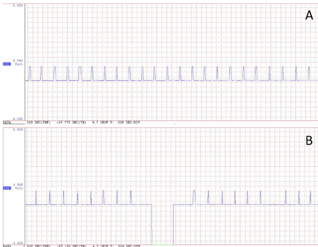
Figure 4. Examples of recorded flight events. Voltage peaks represent complete revolutions of the flight mill's arm. (A) A high quality recording of a flight event with no voltage drops in the recorded signal. (B) A flight event with a voltage drop in the recorded signal. Please click here to view a larger version of this figure.
