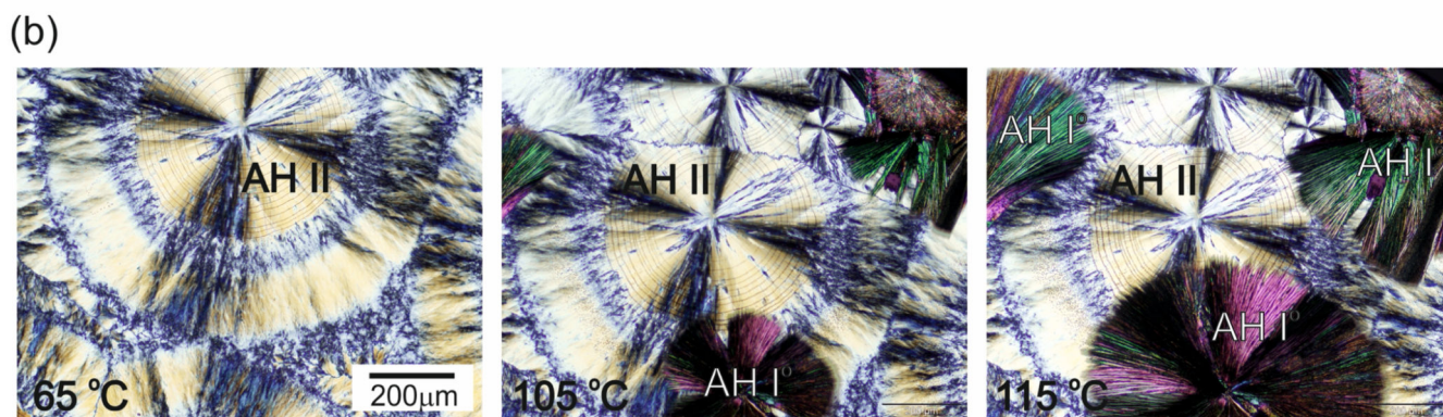
Fig. 6. (a) DSC curves (heating rate 10 °C min -1 ) of 4-AQ anhydrate polymorphs; mp – melting point. The inserts show the glass transition and AH II → AH I° phase transformation. (b) Microphotographs showing the AH II → AH I° phase transformation in the temperature range 105 to 115 °C.
