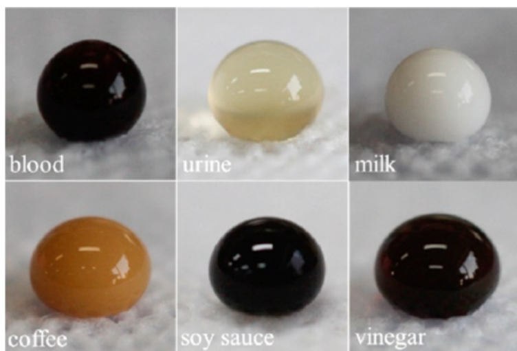
Fig. 7 Digital photographs of various liquid droplets of about 80 \mu\text{L} in volume testing on PP nonwoven fabrics. Reprinted with permission from [85]. Copyright (2015) American Chemical Society
