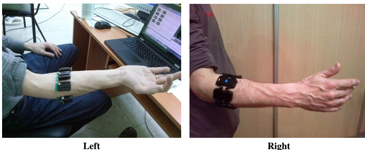
Figure 1. Electrode placement: DELSYS® Trigno™ wireless sensors ( left ) and MYO™ Thalmic bracelet ( right ).
