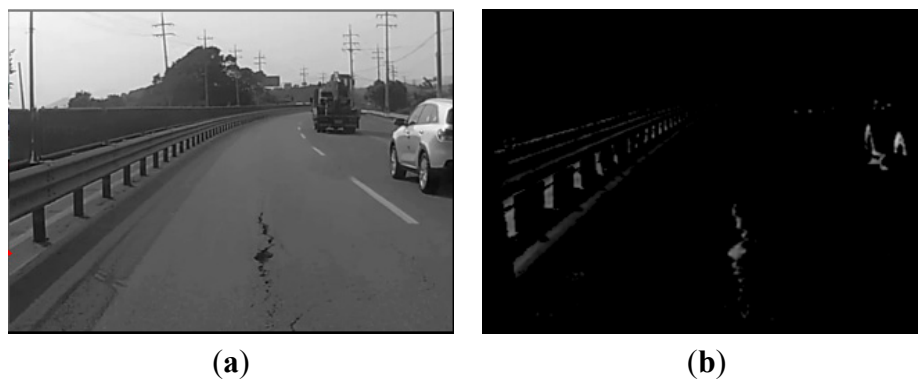
Figure 3. Pre-processing: (a) grayscale conversion; (b) thresholding.
