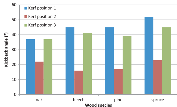
Figure 9. Dependence of kickback angle on kerf arrangement for four wood species.
