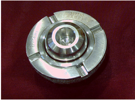
Fig. 1 The bearing used in the current study was the M2a Taper (Biomet, Warsaw, IN, USA), featuring a wrought cobalt-chromium tapered insert that is impacted into a titanium porous plasma spray-coated outer shell and articulated with a wrought cobalt-chromium modular femoral head. Acetabular component outer sizes ranged from 48 mm to 70 mm in 2-mm increments. Available head diameters were 28 mm and 32 mm, each with seven neck length options from -6 to +12 mm. Printed with permission of Joint Implant Surgeons, Inc, New Albany, OH, USA.
