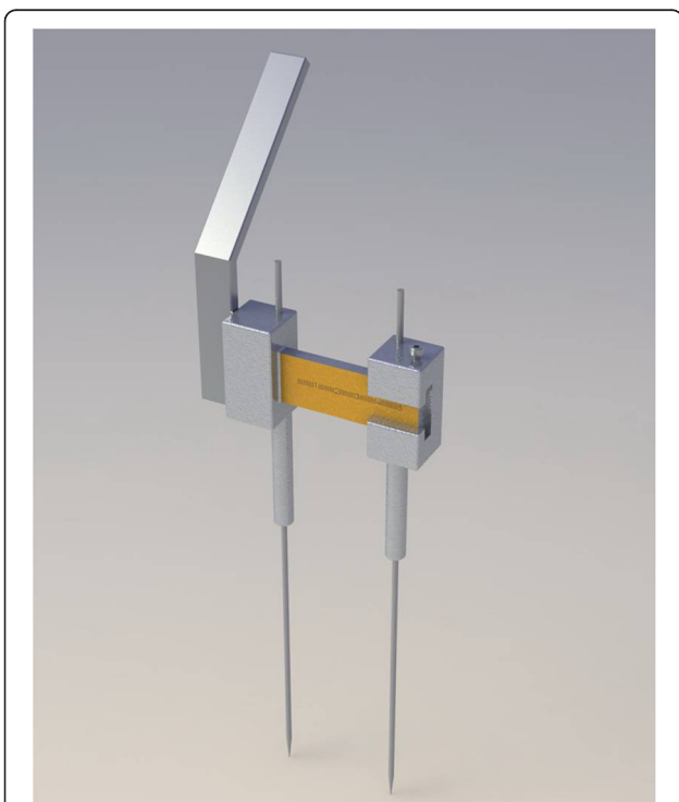
Fig. 1 Three-dimensional model of the new adjustable drill guide prototype
