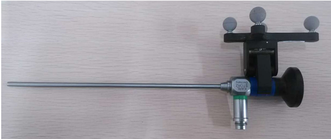
Fig 3. Reflection marker fixed to the endoscope. The marker allows for real-time lens tracking during surgery.
