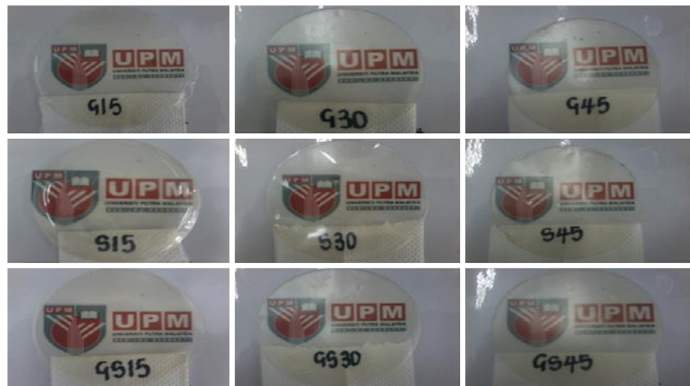
Fig. 2 SPS films prepared using different plasticizer type and concentration
