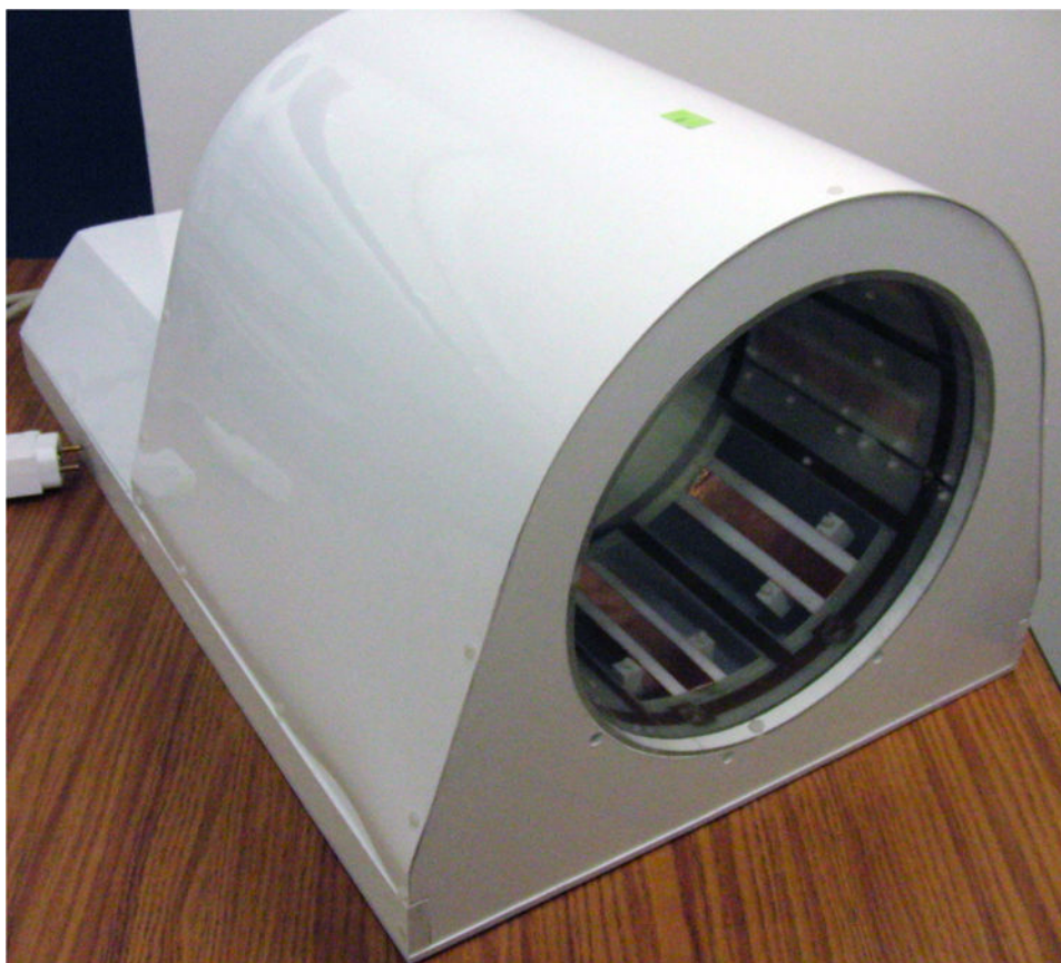
Figure 9. 7 Tesla ^{23}\text{Na} birdcage with coplanar ^1\text{H} striplines visible through the clear interior shell.
