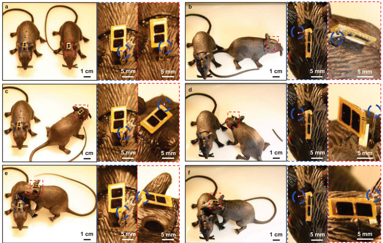
Fig. 7. (a)-(f) Operation of solar powered energy harvesters using model representations of mice ((a), (c), and (e) for H-type harvesters and (b), (d), and (f) for V-type harvesters). These models demonstrate function in situation similar to Figure 4.
