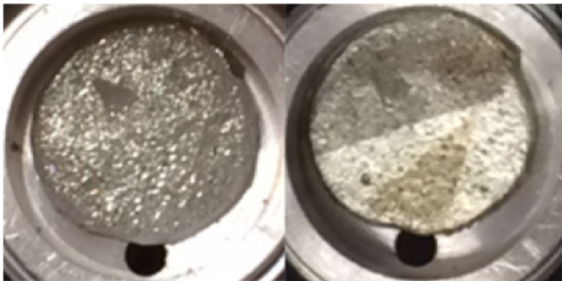
Figure 2. Germanium metal disc in irradiation pocket before (left) and after (right) flowing-liquid-cooled irradiation with 20 \mu\text{A} of 16 MeV protons for 1 h.
