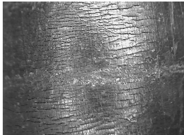
Figure 1. The surface of a used transesophageal echocardiography probe under the microscope during an outbreak: The surface is scratched and broken.
