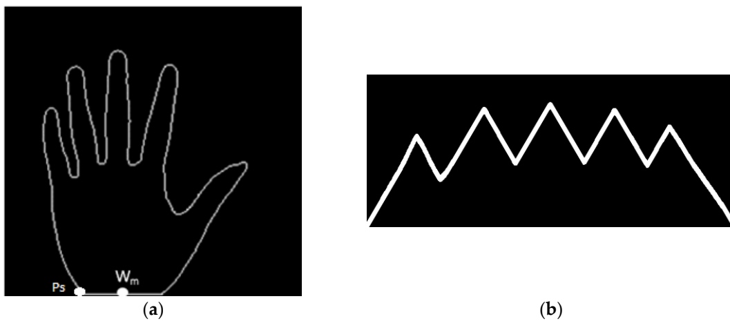
Figure 4. (a) Contours of the palm region; (b) Distance distribution profile of the palm contours constructed using the Euclidean distances between the wrist middle point W_M and palm contour pixels.
