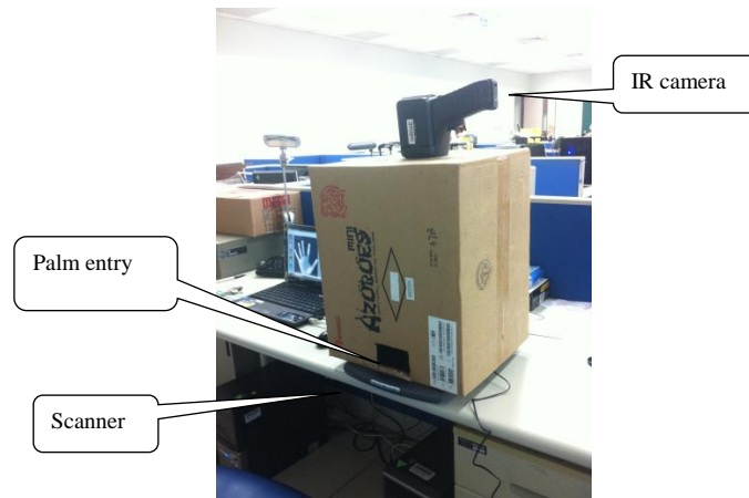
Figure 14. The configuration of the image collection system.
