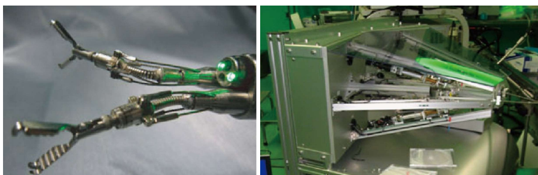
Figure 11 Scorpion like endoscopic robot is an externally mountable robot arms system. It is actuated by external actuators through traction cables (right). Suzuki et al [74] , 2010.
