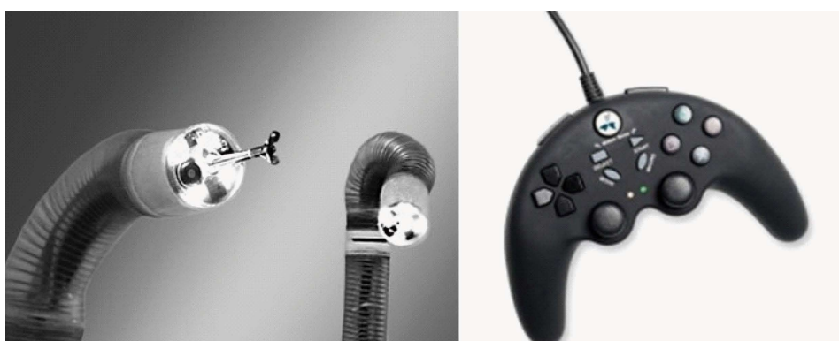
Figure 6 Endotics double balloon probe. Locomotion is executed using the inch-worm mechanism. Courtesy of Endotics SRL, Italy.
