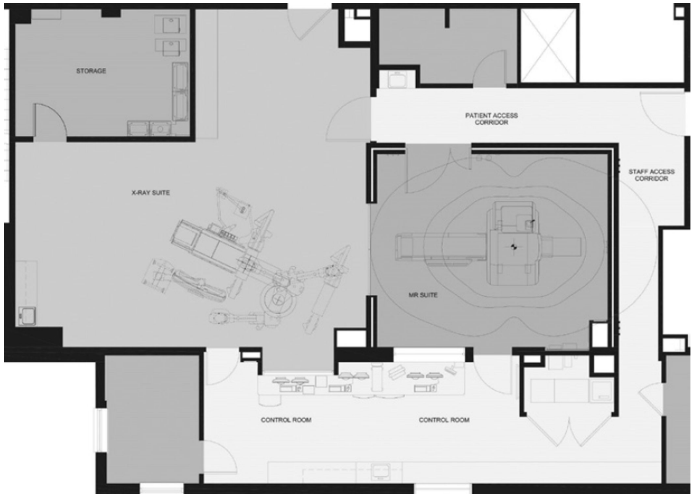
Figure 1. Floor plan of the National Institutes of Health hybrid magnetic resonance (MR) cardiac catheterization lab. Image courtesy of Christopher Dail, project architect, National Heart, Lung, and Blood Institute, Bethesda, MD.
