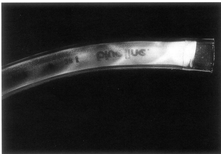
Figure 3 Pattern of powder deposition at the proximal end of the endotracheal tube after multiple actuations from the Turbohaler.
