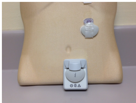
Figure 3. The OmniPod Tubeless Insulin Pump with a pod (right) and a handheld device that functions as a blood glucose meter and communicates wirelessly with the pod to deliver insulin based on the patient's personal settings.
