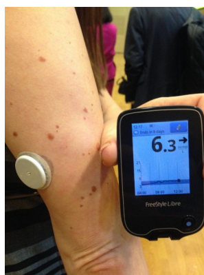
Figure 8. The Abbott FreeStyle Libre Flash Glucose Monitoring System (available online: http://diatribe.org/issues/69/new-now-next/1 , accessed on 3 December 2015).
