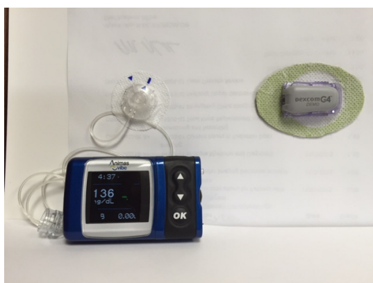
Figure 7. The Dexcom G4 Continuous Glucose Monitoring System (left) displays readings and graph on the screen of the Animas Vibe Insulin Pump.
