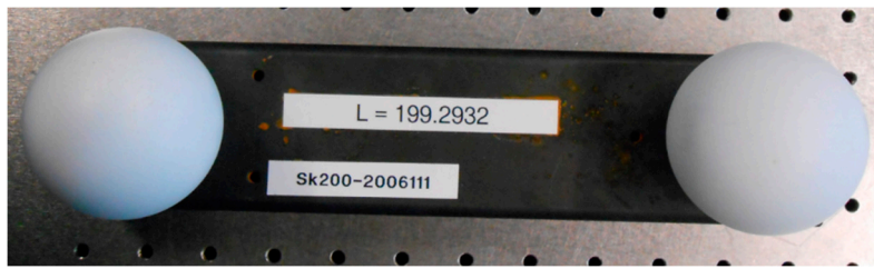
Figure 3. Specimen for calibration: calibrated ball bar.
