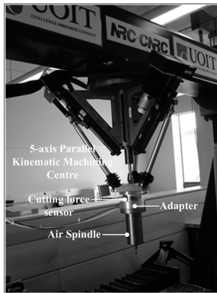
Figure 1. Experimental setup for implementing the sensor system for cutting force measurement.
