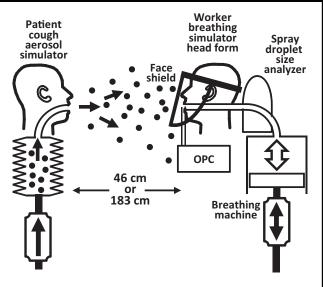
**FIGURE 1**. Schematic of the experiment using particle spectrometers. The mouth of the cough aerosol simulator and the mouth of the breathing simulator were 152 cm (60 inches) above the floor and 46 cm (18 inches) or 183 cm (72 inches) apart. For experiments using influenza virus, the optical particle counters (OPCs) and the droplet size analyzer were not used, and a respirator was sealed to the breathing head form to act as a filter to collect the virus that was inhaled.
