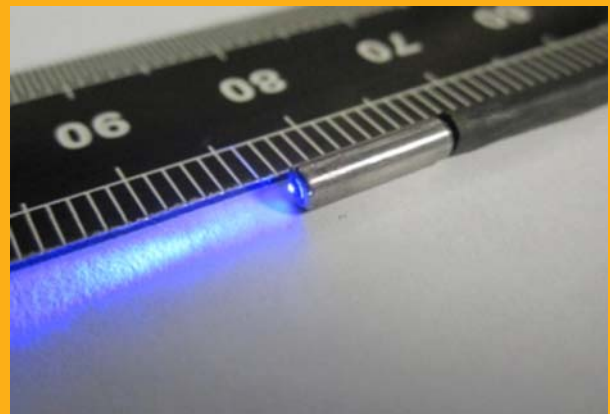
Photo of ~2.3 mm diameter flexible endoscope distal tip.
