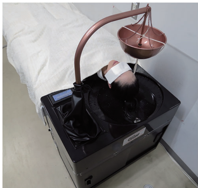
FIG. 3. Shirodhara robotic oil-drip system. The liquid was warmed and circulated inside the system and poured on the forehead of the subject through a bundle of cotton strings attached under the nozzle. The ends of the strings were set 8 cm above the forehead. Temperature, pattern, and flow speed can be specified. Color images available online at www.liebertpub.com/acm
