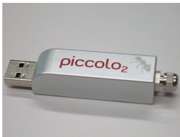
Figure 3. Fiber optic decay time-based O_2 sensor with an USB interface and (on the right side) a standard fiber connector. The fiber and its 20- \mu\text{m} tip (coated with a polymer incorporating a quenchable oxygen indicator) are not shown. © PyroScience GmbH.
