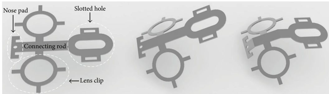
FIGURE 2: A schematic of the spectacle frame showing the functional components including the slotted hole, lens clip, nose pad, and connecting rod. And a brief visualization of the 3D shape is present.
