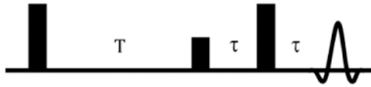
Figure 2. Inversion Recovery with Electron Spin Echo readout (IRESE) pulse sequence
