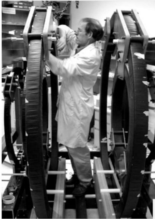
Figure 1. Main magnet for EPR O 2 imaging with a human subject.
