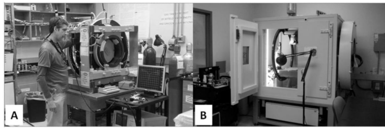
Fig. 3. A. 250 MHz pulse Electron Paramagnetic Resonance oxygen imager. B. Precision X-ray XRAD225Cx image-guided biologic irradiator/CT imager.
