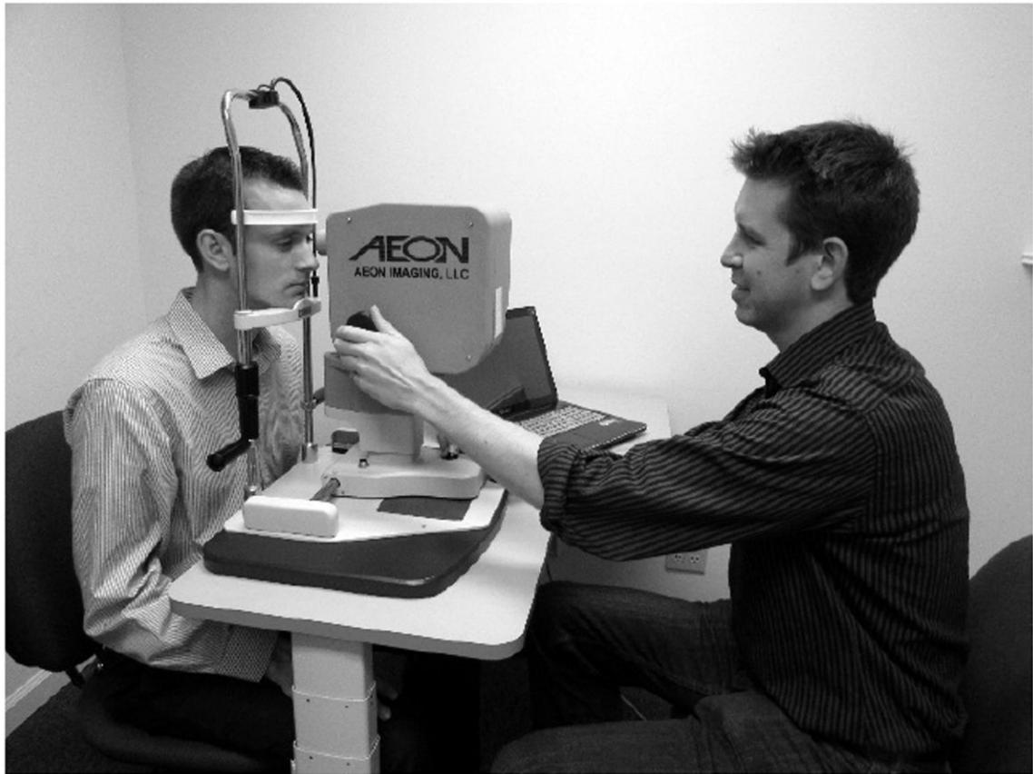
Figure 7. The Digital Light Ophthalmoscope (DLO), mounted on a slit-lamp alignment base for retinal imaging.
