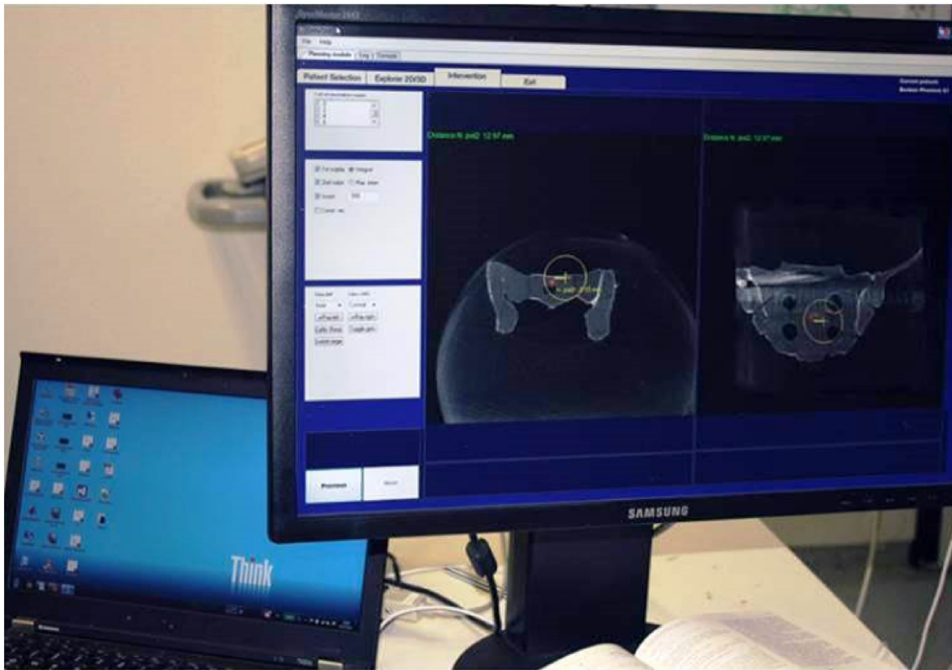
Fig 5. EM navigation. Illustration of the EM navigation software during k-wire positioning.
