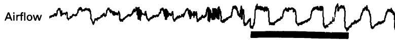
Nasal airflow in a patient receiving continuous positive airway pressure (CPAP) treatment. The underlined breaths are "chopped off" – that is, they lack the normal rounded contour seen in the normal breath at the extreme right and are caused when subcritical levels of CPAP are used, resulting in residual partial upper airway obstruction.
