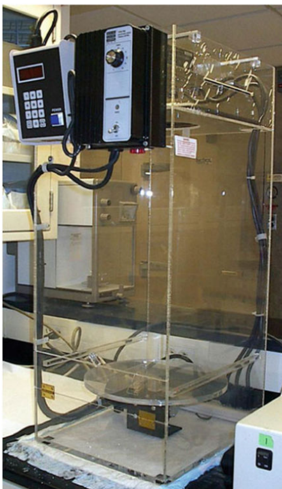
Fig. 2. Specialized UV delivery device created to deliver a specific damaging dosage of UV-C light. The machine consists of three appropriate UV bulbs, a turntable and timed shutter, all enclosed by plexiglass. The distance from the bulbs to the sample (3 ft) determines the amount of damage the bulbs can give over a set time
