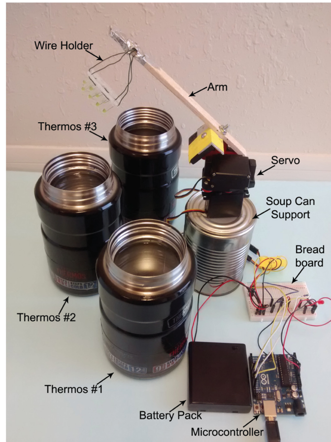
Fig 1. Setup of the low-cost and rapid TTC. Major components include three 24-oz thermoses and a pan-and-tilt servo set to control the up, down, and rotational motion to shuttle PCR vessels in and out of the thermoses. Also included are the battery pack, the Arduino electronic controller, and a breadboard. To reduce costs, the pan-and-tilt setup is constructed using a soup can for a fixed height, a wood stick, and a PCR tube holder made with metal wire.
