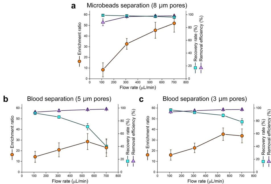
FIG. 5. Separation performance for different flow rates and pore sizes. (a) Results for microbeads separation using  $8 \mu\text{m}$  pores, (b) results for whole blood separation using  $5 \mu\text{m}$  pores, (c) results for whole blood separation using  $3 \mu\text{m}$  pores. Error bars represent standard deviations of 5 different trials.
