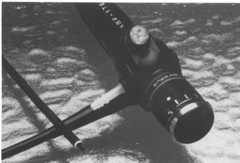
Prototype fibreoptic bronchoscope (Olympus) with insulated/electrically grounded inner sheath (white tip visible) and insulated ball probe catheter protruding out of the suction channel. This monopolar ball probe can be used to coagulate tumour base along the bronchial wall by gentle palpation manoeuvres.
