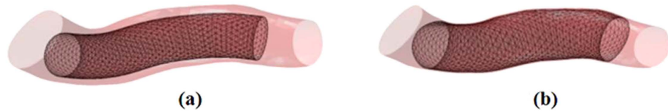
Figure 7. The stent contour before and after the expansion. (a) Initial stent contour. (b) Final stent contour satisfying the termination conditions.
