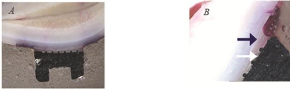
Fig. 3. Stereomicroscopic views (A and B) of a sample sectioned in mesiodistal direction (black arrow: enamel-adhesive interface, white arrow: adhesive-bracket interface)
