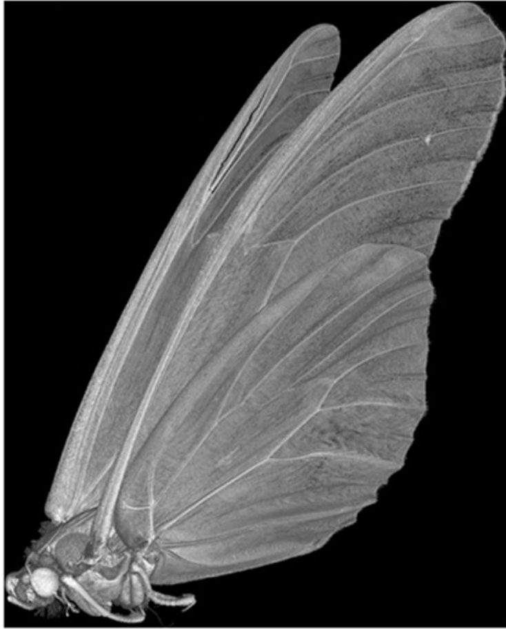
Figure 4. A butterfly scanned at 15 \mu\text{m} voxel size, 70 kV, 570 \mu\text{A} , 1000 ms exposure time and a scan length of approximately 9h.
