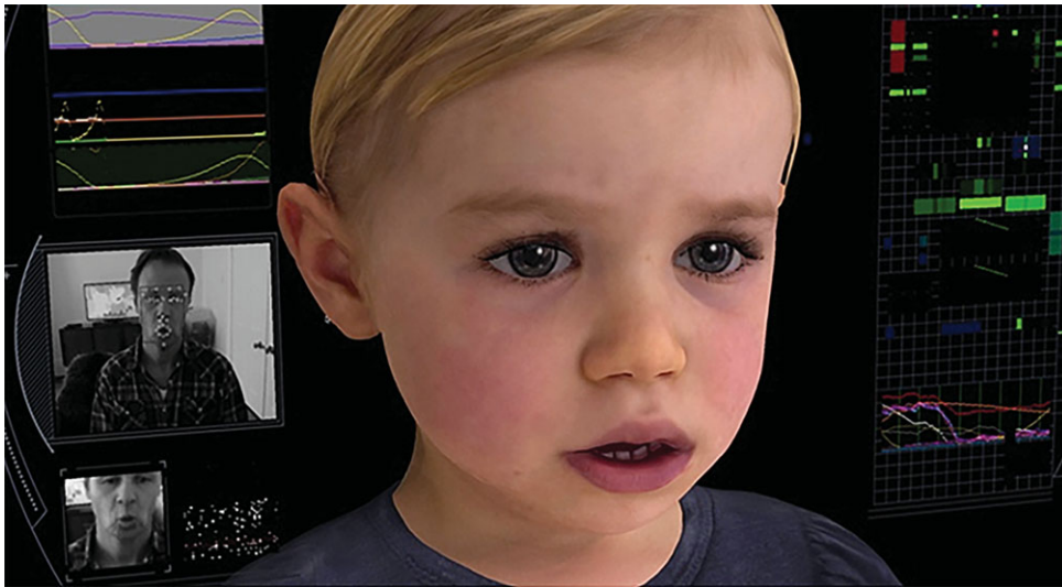
Figure 2. BabyX (v. 3). Sensorimotor online learning session screenshot in which multiple inputs and outputs of the model can be viewed simultaneously including: scrolling displays, spike rasters, plasticity, activity of specific neurons, camera input, animated output.
