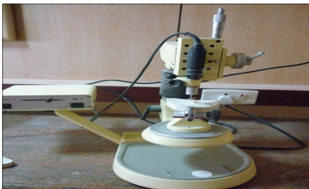
Figure 2: Sample preparation using milling unit
