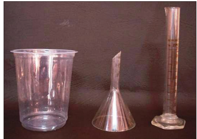
Figure 2: Armamentarium used in this study (disposable glass, glass funnel, and graduated measuring jar)
