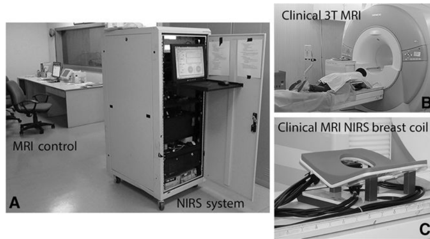
Figure 1. An overview of the MRI/optical system. The optical system is housed in the MRI control room (A) and light is piped into the MRI suite for patient imaging using fiber optic cables (B). A combined MRI/optical breast coil (C) makes simultaneous MRI and optical imaging possible.
